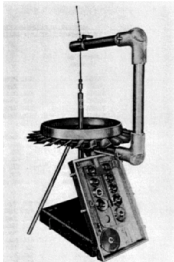
Figure 1-5. Typical Balance Checking Set-up – Helicopter Engine Fan Assembly
