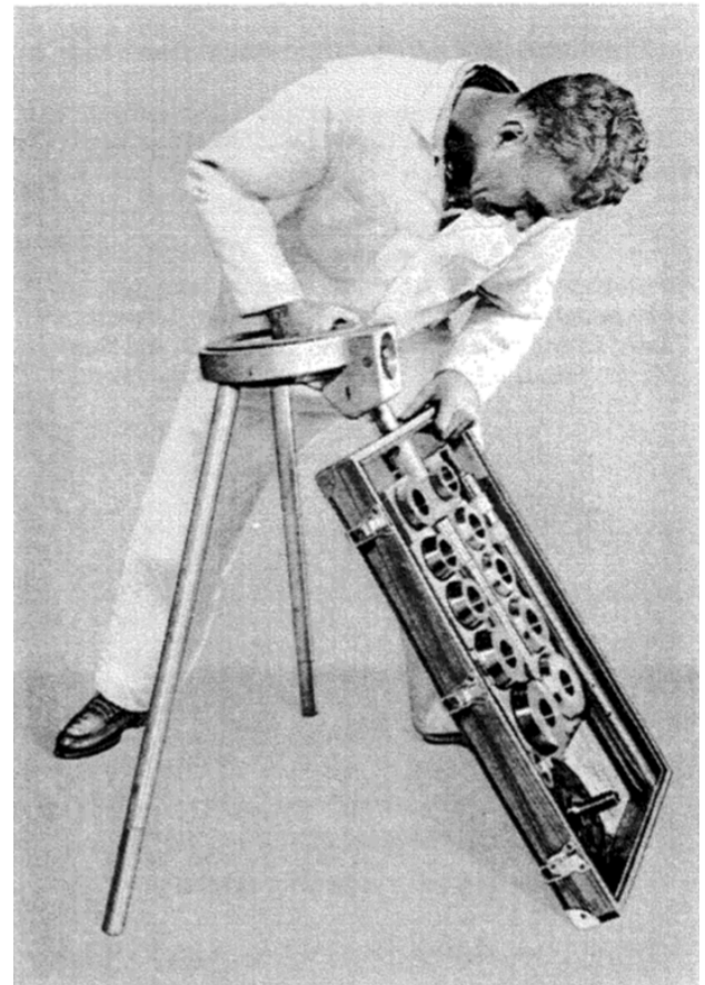
Figure 3-4. Assembling Work Stand Casting to Bottom Half of Storage Case.
